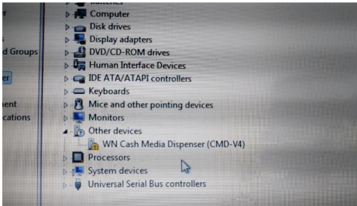
Figure 9. ATM dispenser connected to a computer without the necessary drivers
